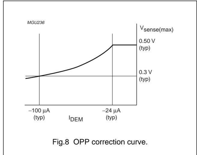
Fig.8 OPP correction curve.
