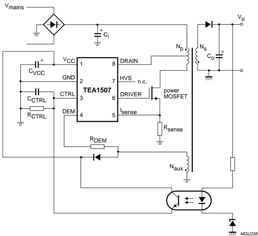
Fig.10 Flyback configuration with secondary sensing.
