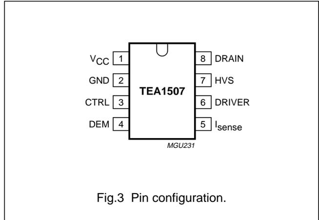
Fig.3 Pin configuration.
