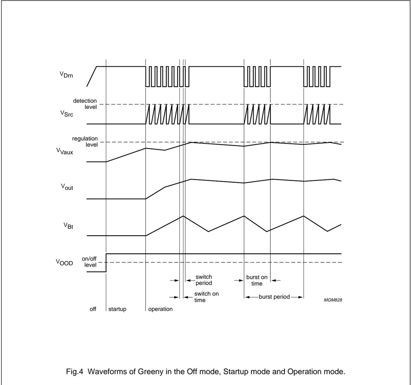
Fig.4 Waveforms of Greeny in the Off mode, Startup mode and Operation mode.
