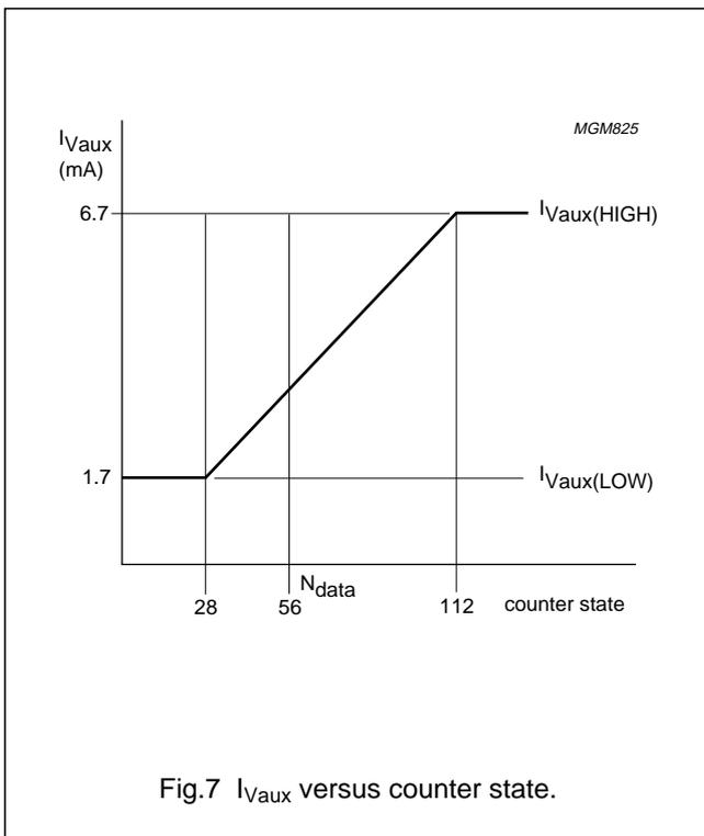
Fig.7  $I_{V_{aux}}$  versus counter state.
