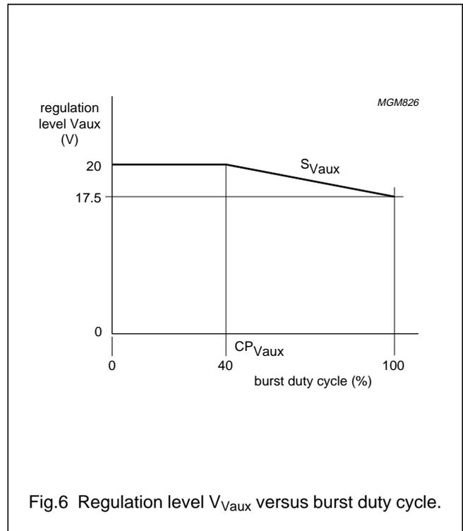
Fig.6 Regulation level  $V_{Vaux}$  versus burst duty cycle.
