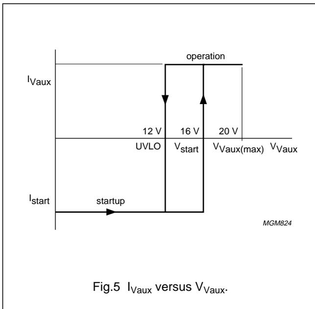
Fig.5  $I_{Vaux}$  versus  $V_{Vaux}$ .
