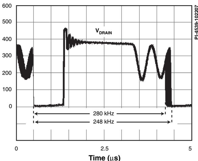
Figure 4. Frequency Jitter.
