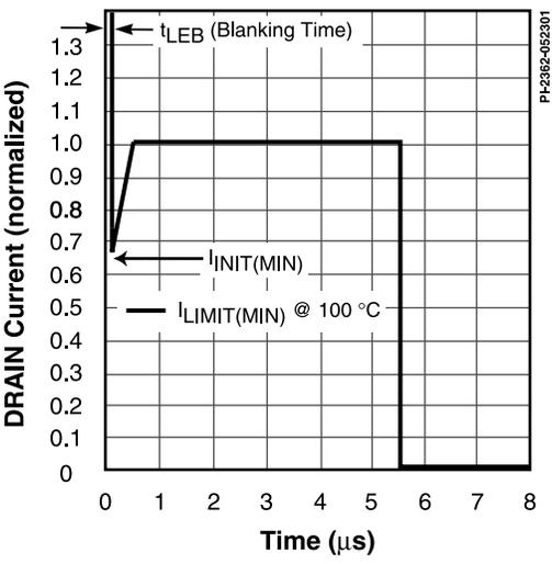
Figure 20. Current Limit Envelope at  $f_{osc} = 132$  kHz.
