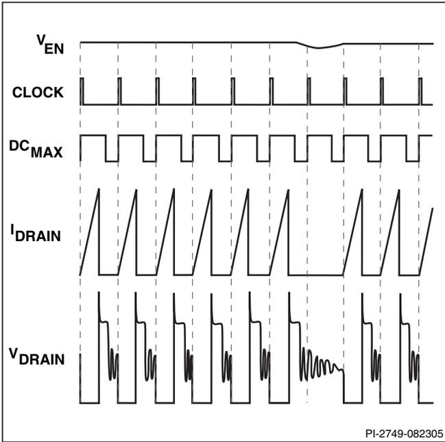
Figure 6. Operation at Near Maximum Loading ( $f_{osc}$  264 kHz).
