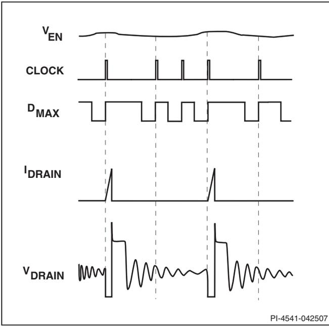
Figure 9. Operation at Very Light Load ( $f_{osc}$  132 kHz).
