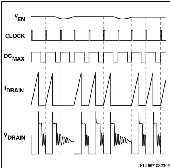
Figure 7. Operation at Moderately Heavy Loading ( $f_{osc}$  264 kHz).
